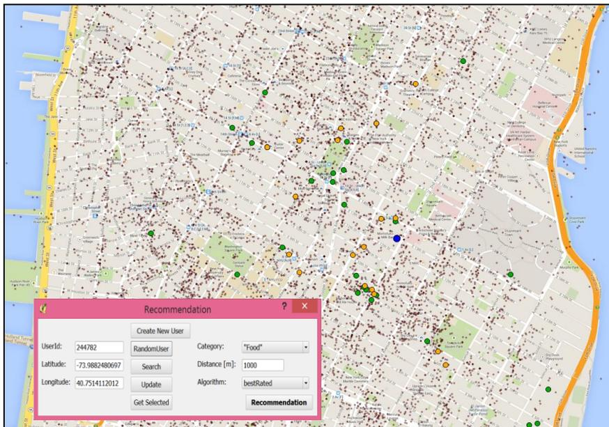
Figure 2 shows the deviation of recommendations and visited locations for user 1977211 in QGIS and the interface of the plug-in. The User-location is the blue point in the center. Visited Locations are represented by green points. Recommended locations are orange. Locations are visualized in red, slightly transparent and with smaller points.
