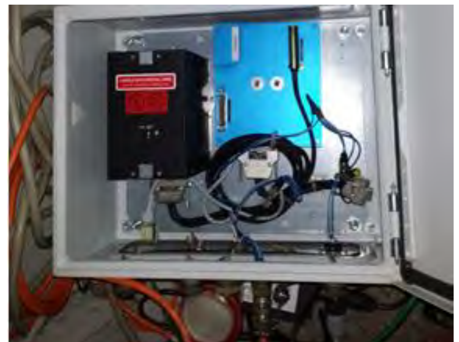
The box including Gyrocompass blue box to process the data
