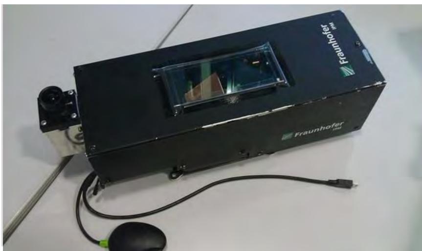
*Fraunhofer UAV-Scanner with the camera for VO*
